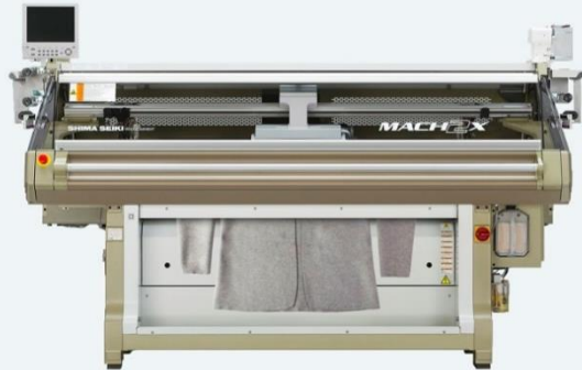
3D kötőgép (Ministry of Supply's '3D Print-Knit')
